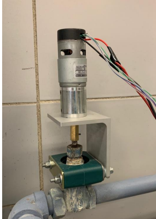
Figure 5. Final motor mount design
